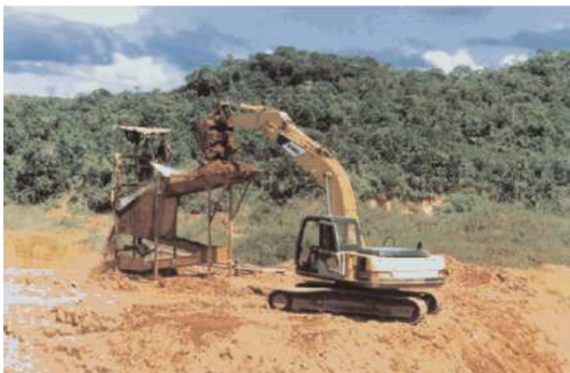
Picture 14: Washing of the substratum and passing it through the chute with mercury to catch gold
